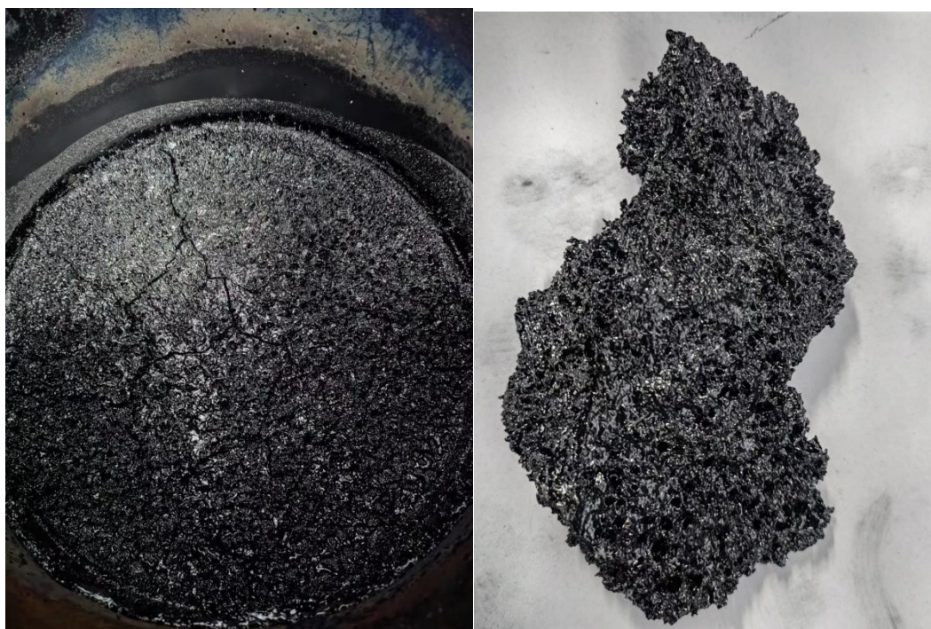
Figure 1. Laboratory-scale co-coking coke produced from low-ash coal and vacuum residue.
